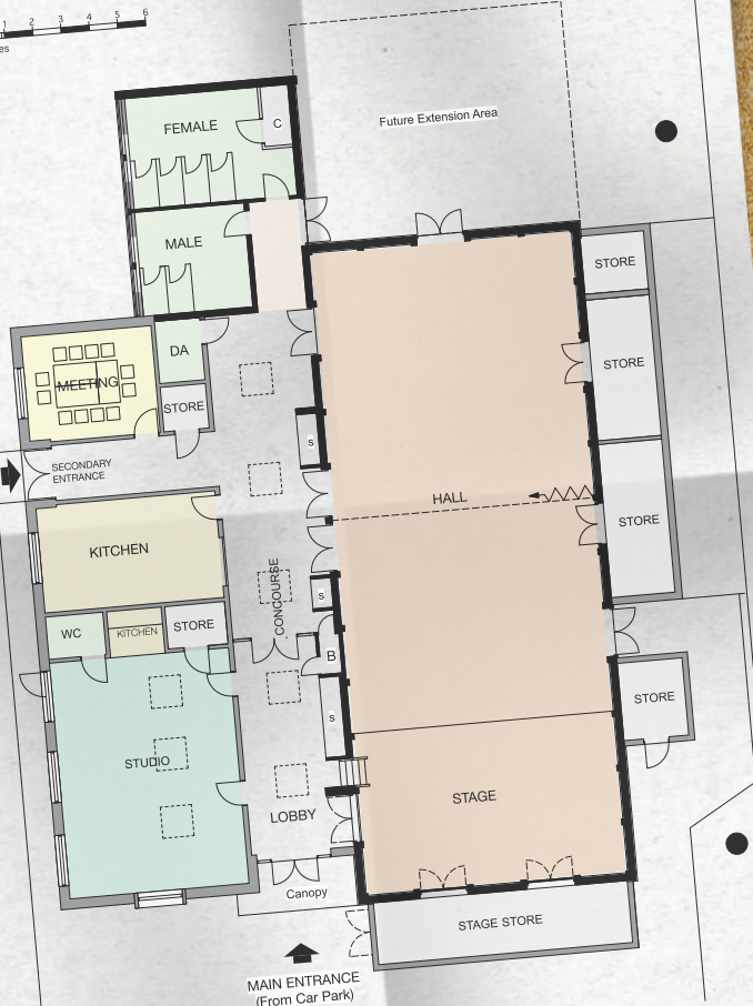
FLOOR PLAN HAGLEY COMMUNITY CENTRE EXTENSIONS / REFURBISHMENT
